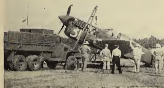
Colonel Reed's portable hoist lifts a wrecked P-40.
